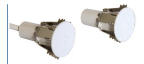
Typical applications include: armoured doors, iron doors and gates. It is pressure mounted into a 22 mm diameter hole. The reed section contains a tight reed bulb with polyurethane resin and an anti-tampering loop to reduce violation risks.
